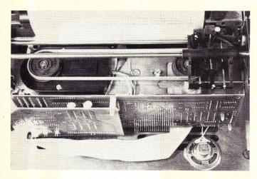
Photo 1. With the cover off, the simplicity of the Comprint mechanism is revealed. The oval belt slides the stylus head past the paper, which is friction-fed continuously during printing. When the printer is idle, the printhead is to the right.
